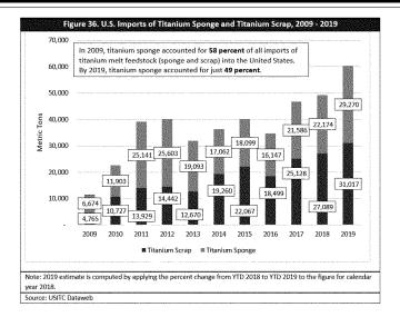
Increased use of titanium scrap as feedstock does not, however, eliminate the need for new titanium sponge. In the United States, scrap accounts for approximately 59–66 percent of titanium melt feedstock. <sup>108</sup> Using scrap as a source of feedstock allows titanium manufacturers to offset price increases in sponge with increased consumption of scrap, or vice-versa. <sup>109</sup> However, the chemical composition requirements for aerospace rotating-grade titanium
