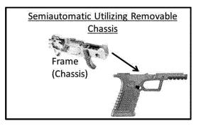
(iv) *Certain locking block rail system semiautomatic pistols:* the internal removable frame of the pistol that provides housing for the trigger mechanism, and a structure designed to integrate the slide rails, provided a portion is partially exposed to the exterior to allow identification.
