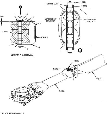
1. DLADE RETWININ BOLT 2. THRUST WASHER 3. CAM HANDLE 4. SPRING CLIP 5. HEX NUT 6. LOCK RING 7. O-RING 8. RETAINER 9. PITCHCASE 10. FLEXBEAM 11. MAIN ROTOR BLADE
