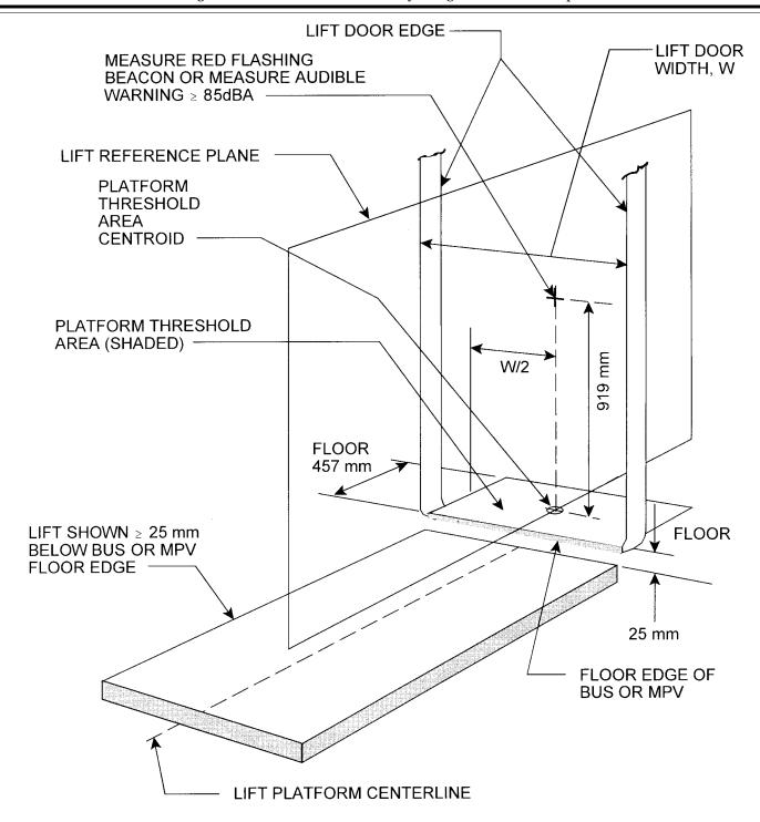
PLATFORM THRESHOLD AREA AUDIBLE WARNING MEASUREMENT POINT (\$5.1.2.4)
