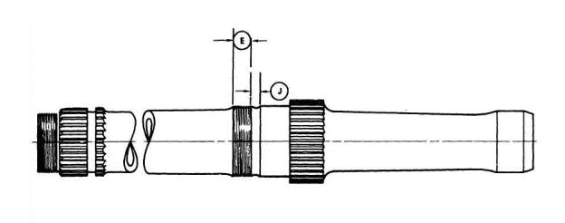
(2) If there is a crack, pitting, or corrosion, before further flight, replace the mast with an airworthy mast.
