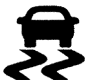
Figure 5: ESC Malfunction Telltale Symbol in FMVSS No. 101
