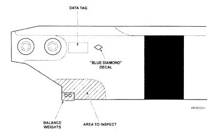
Figure 1. Tail rotor blade inspection.
